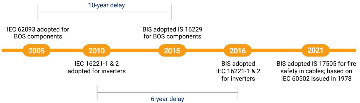
In absence of clear technical standards and certification regime, BOS components, including transformers, junction boxes, cables, mounting structures, module cleaning systems, earthing and lightning systems bear most of the brunt of cost cutting. It has been shown by several studies that faulty BOS equipment selection and installation, accounting for around 30% of solar project cost, has a disproportionate impact on power output.
