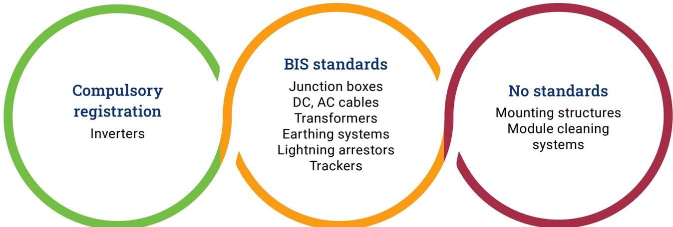
Developers increasingly adopt new and emerging technologies, like robotic module cleaning systems and trackers, to reduce levelised cost of energy. However, there is a significant lag (up to 10 years) in Bureau of Indian Standards (BIS) adopting technical standards for these equipment issued by international agencies like International Electrotechnical Commission (IEC).
